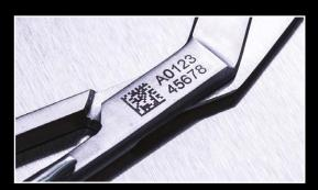
When printed small holes are made in the tape that allows the etching chemical to permeate through the tape. When an etching pad is placed over the tape and pushed onto the metallic item, an electrical circuit is completed. The metal then discolours and is permanently marked with serial numbers or other required information.
