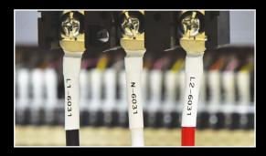
This special non-adhesive tape is made of a special material that is wound in the tape cassette as a flat tube. Once printed with the relevant identification details, the tube is opened up and passed over a cable or terminating connector. Once heated using a heat gun, the tube shrinks to about half its original width, and in doing so grips the cable.
